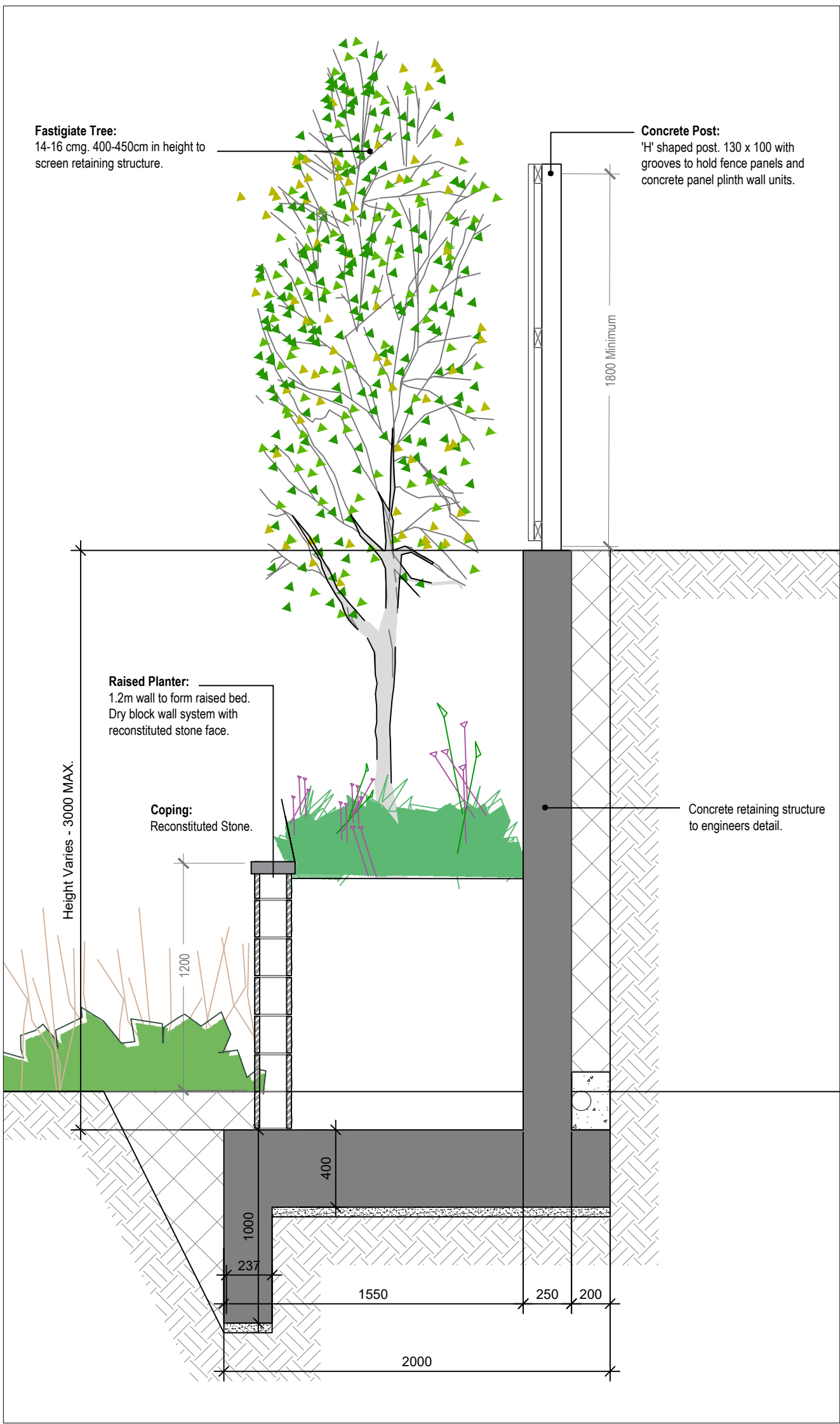
D06 107 Detail of 2.0m high concrete post and timber panel fence on top of retaining structure. scale 1:25
